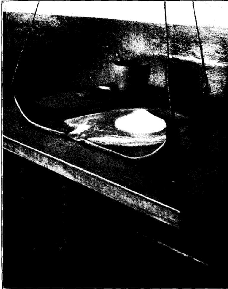
FIGURE 96. Manufacture of Detonators. (Courtesy Hercules Powder Company.) The safe mixing of the primary explosive charge for blasting caps is accomplished mechanically behind a concrete barricade by lifting slowly and then lowering first one corner of the triangular rubber tray, then the next corner, then the next, and so on. In the background, the rubber bowl or box in which the mixed explosive is carried to the building where it is loaded into caps.
