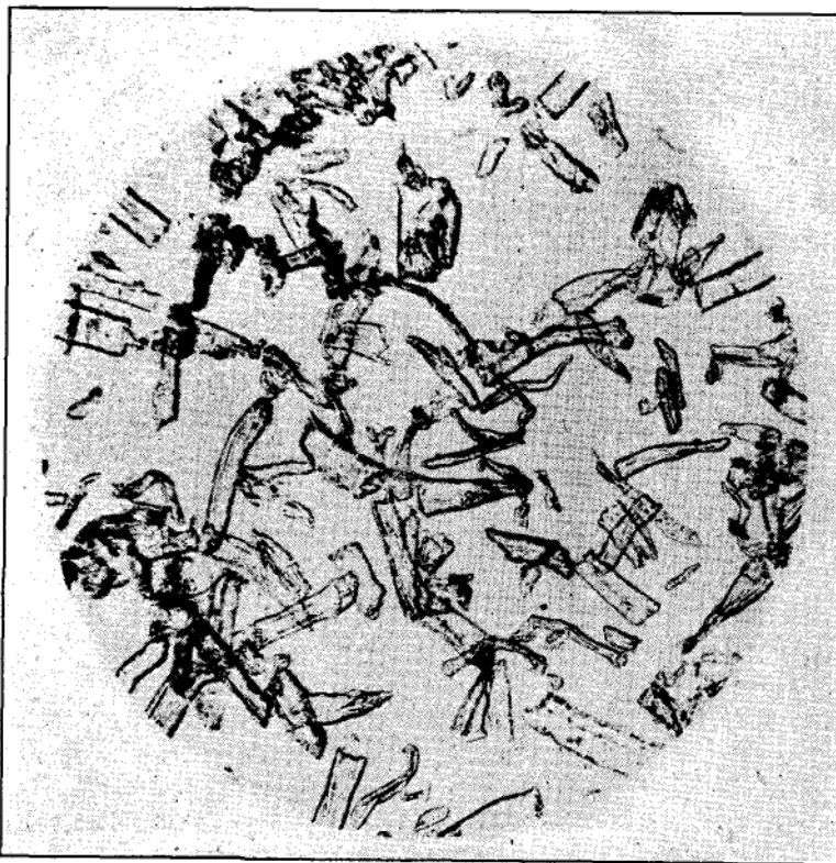
FIGURE 63. Nitrocellulose Fibers after Beating (132X). (Courtesy Western Cartridge Company.)
