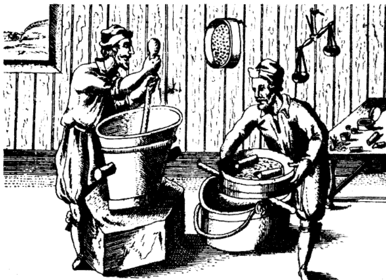
FIGURE 18. Gunpowder Manufacture, Lorrain, 1630. After the materials had been intimately ground together in the mortar, the mixture was moistened with water, or with a solution of camphor in brandy, or with other material, and formed into grains by rubbing through a sieve.
