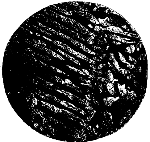
PHOTOGRAPH 12. CUPRO-ALUMINIUM. FORGED AND SUBSEQUENTLY QUENCHED FROM 600°. ×225.
