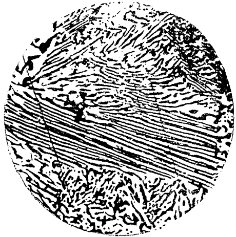
PHOTOGRAPH B. EUTECTIC STRUCTURE. ETCHED WITH ALCOHOLIC FERRIC CHLORIDE. × 870. (Portevin.)
