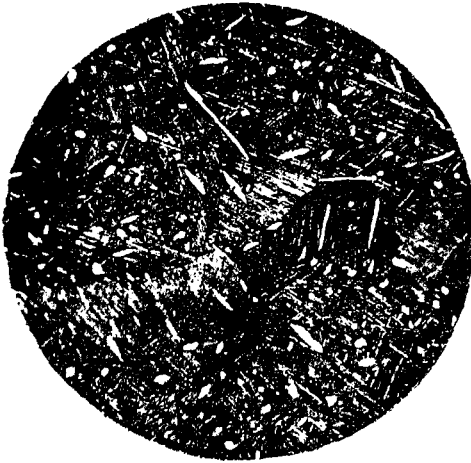
PHOTOGRAPH 13. CUPRO-ALUMINIUM. FORGED AND SUBSEQUENTLY QUENCHED FROM 700°. × 60. (Brenil.)
