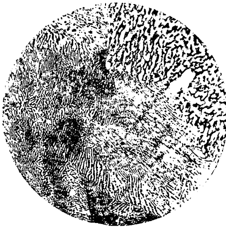
PHOTOGRAPH A. EUTECTIC STRUCTURE. ETCHED WITH ALCOHOLIC FERRIC CHLORIDE. × 500. (Portevin.)
